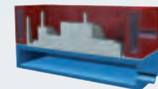
Place the moulding box onto the pattern
