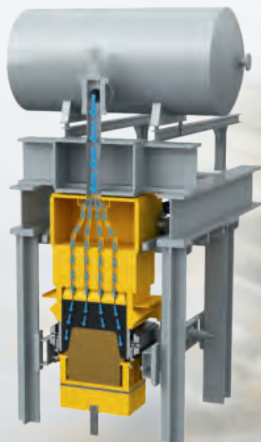
SEIATSU airflow pre-compaction process
