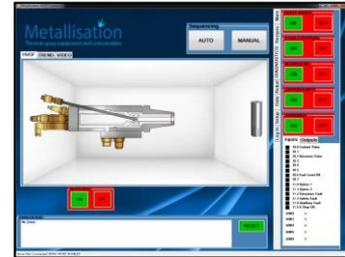
All typical spray parameters are monitored and a **trending** screen is included. This enables the system to check that operation remains within expected limits and report if the system strays outside of these limits during operation.
