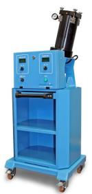
The 2007MF-PF-HC powder feeder is a positive displacement feeder which uses an offset disc that rotates and collects powder in small holes. At a certain point powder is blown from the holes into the powder feed line where the Argon gas carries the powder through the powder feed hose to the required point of exit.
