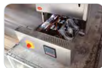
Pull out drawer with electro components for easy service access
