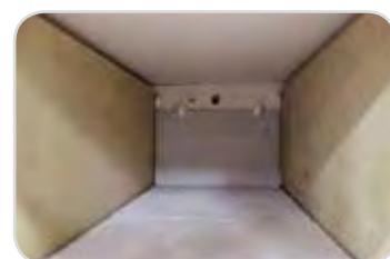
Furnace chamber with thermocouple and ventilation chimney
